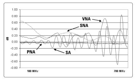
Figure 6. Conversion loss airline delta instrument comparison.
