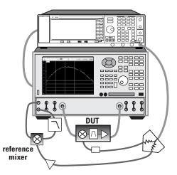
Figure 13. PNA group delay configuration using the vector-mixer calibration.
