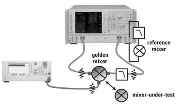
Figure 10. 8720ES group delay configuration using golden and reference mixers.
