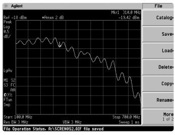
Figure 4. Output-power measurement of a mixer using the configuration illustrated in Figure 1.
