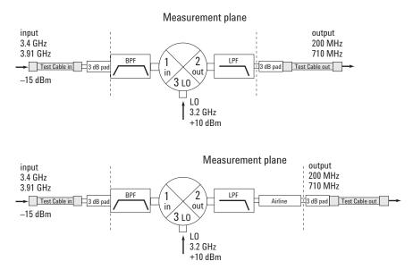
Figure 9. Converter configuration for airline delta comparison.
