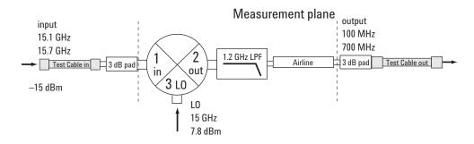
Figure 2. Example of a mixer-under-test with addition of airline.
